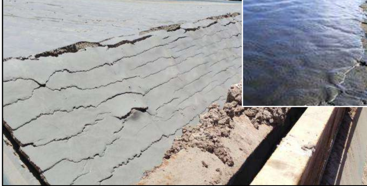
Slurry tailings: solids content \approx 20-40%
