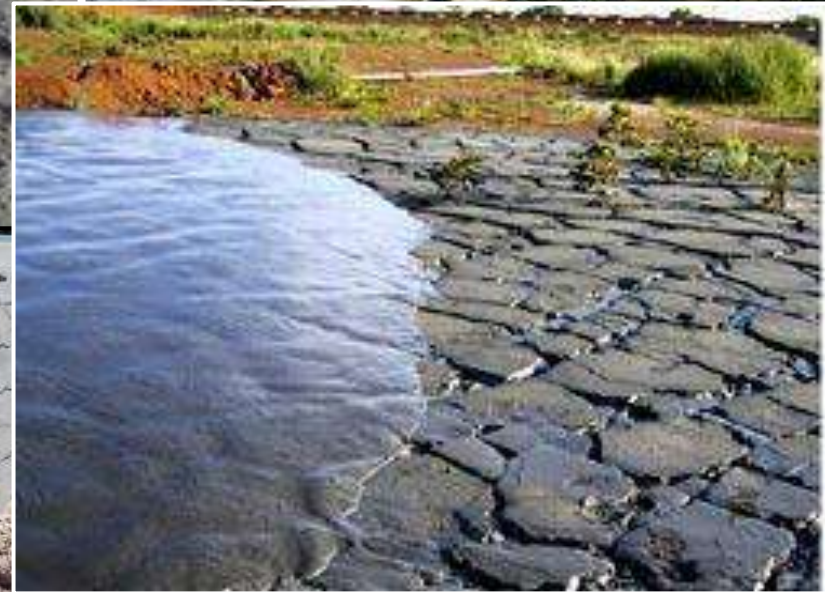
Thickened and paste tailings: solids contents 40-70%, 70- 75%
